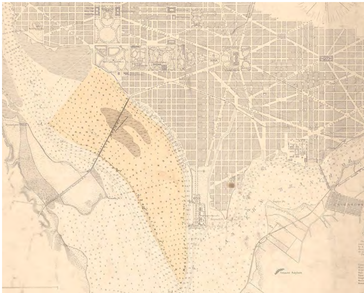
Fig. 9: 1882 Map of Washington and Georgetown Harbors showing visible accumulation of sediment below the Long Bridge. (Library of Congress)
