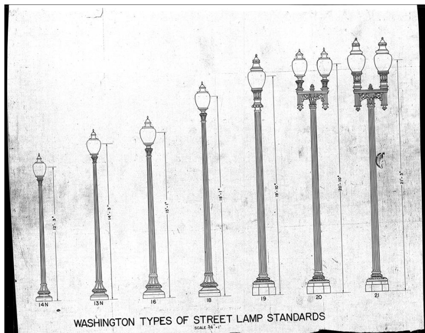
Fig. 103: By the time this drawing was prepared in 1930, the OPBPP had standardized what lampposts were used in the cultural landscape. These were limited to Washington Standard and Twin Twenty units of various sizes. (National Park Service 1930)
