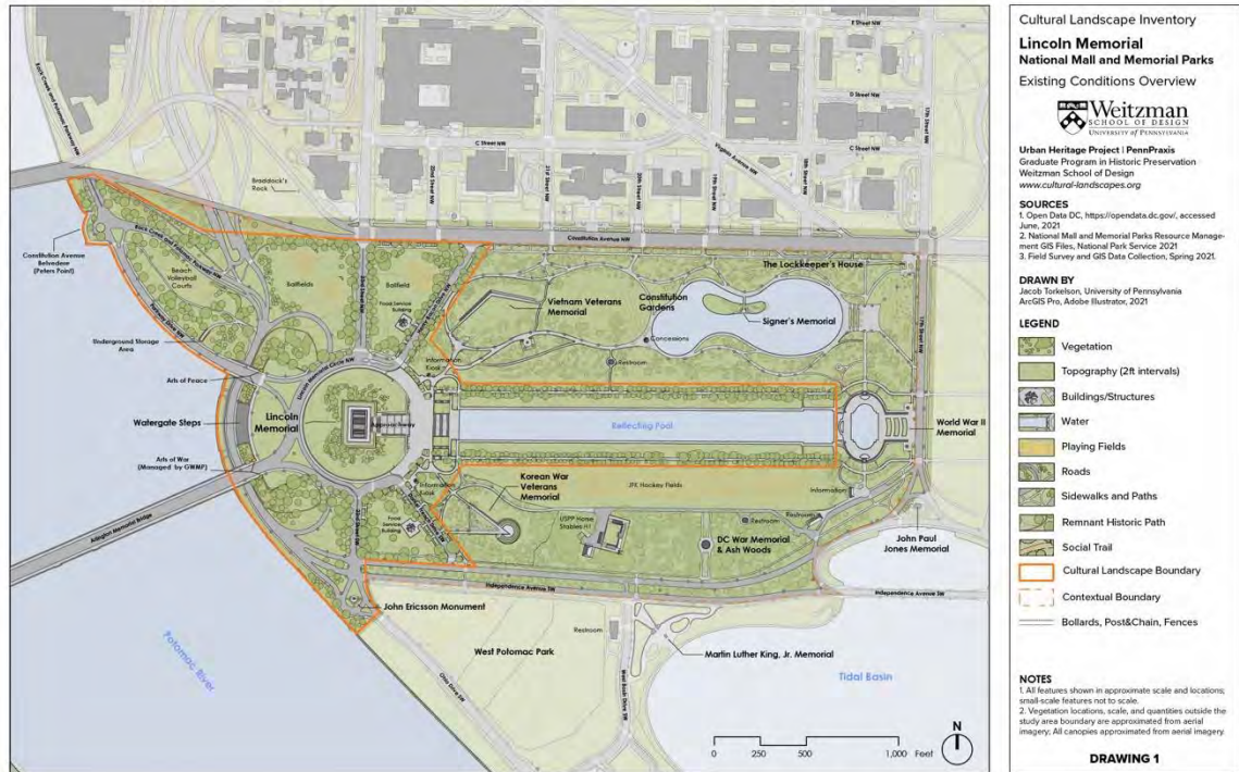
Fig. 1: Existing conditions site plan of the Lincoln Memorial cultural landscape. The cultural landscape boundary is shown in solid orange and the contextual boundary is shown in dashed orange. Full size drawings are located at the end of this report. (Torkelson 2021)
