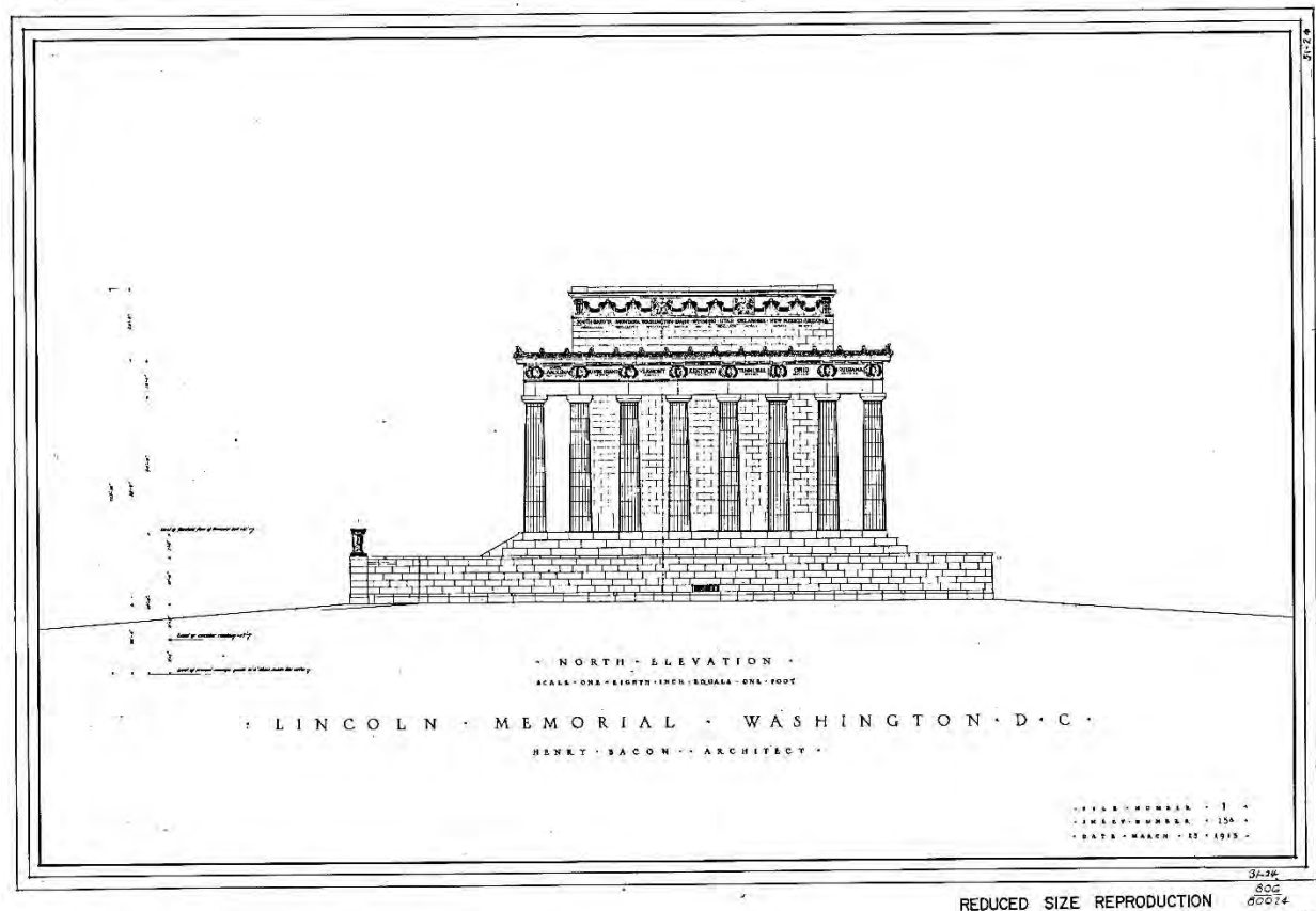
Fig. 24: North elevation drawing for the Lincoln Memorial structure, as of 1915. (Bacon 1915d)
