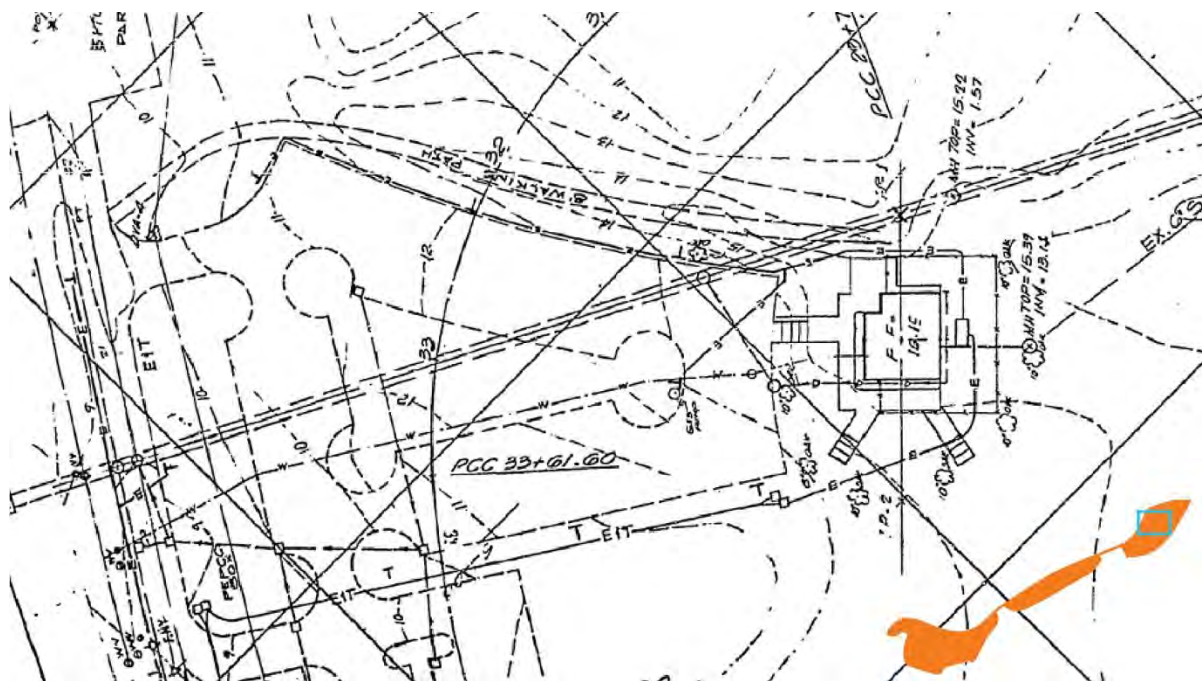
FIGURE 62: This existing conditions drawing of Section E from 1976 shows the circulation features around the 1961 golf center. They include three ramps with stairs, a short path along the driving range area, and a keyhole-shaped parking lot. The location of the excerpted drawing is shown by a blue square on the orange locator map in the lower right corner. (Excerpt from Sheet 6, ETIC 831_41018A)
