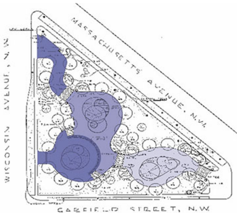
Diagram of the four terraces that organize the cultural landscape's spatial arrangement, from the highest-elevation terraces (dark blue) to the central terrace, to the lowest-elevation terrace (light blue). Diagram overlaid on the 1963 landscape plan for Bryce Park, as designed by NPS Landscape Architect William Belden. (Belden 1963)
