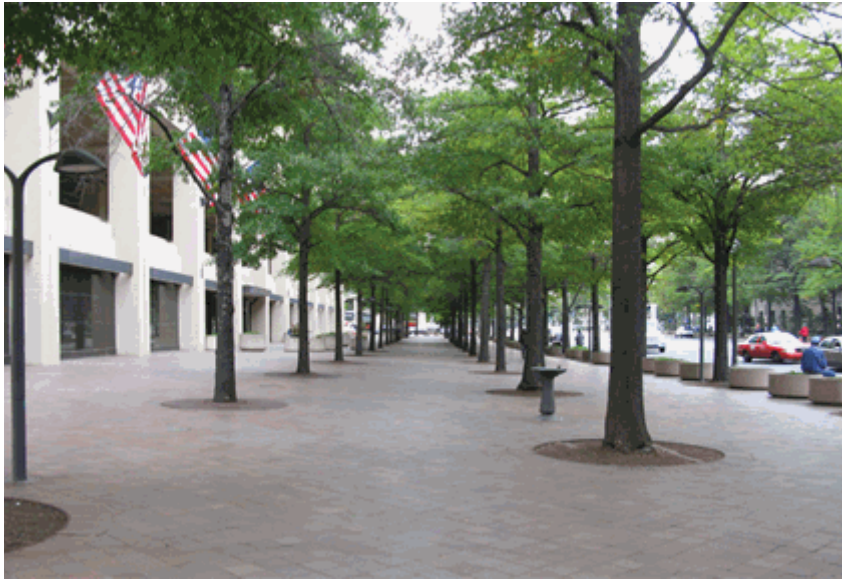
Between 9th and 13th Streets, and in front of the Canadian Embassy, the sidewalk is 30 feet wide allowing for a third row of trees. This image illustrates the width of the sidewalk in the block occupied by the J. Edgar Hoover Building.
